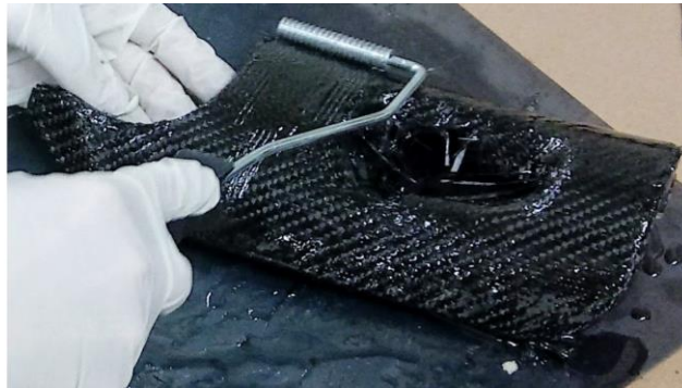
Figure 43. Smoothing out air pockets.
