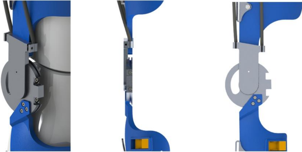
Figure 14. Minimization of profile at the knee joint.
