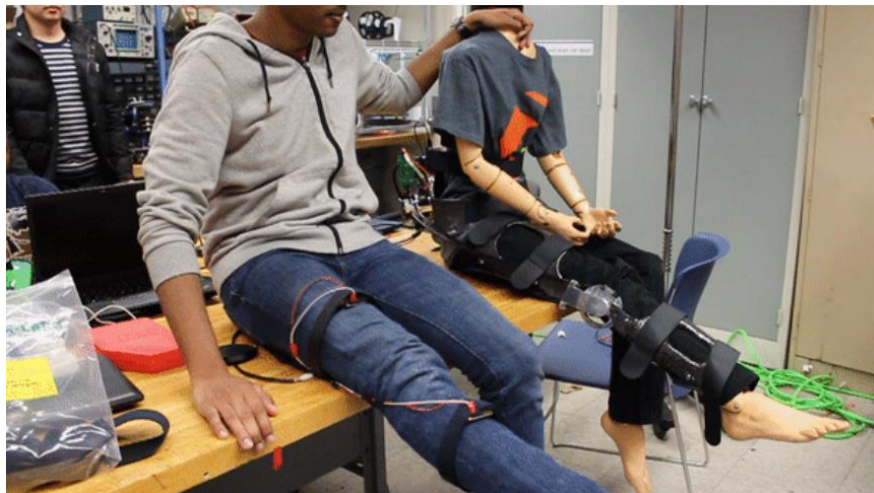
Figure 53. Testing of the control system using a mannequin.
