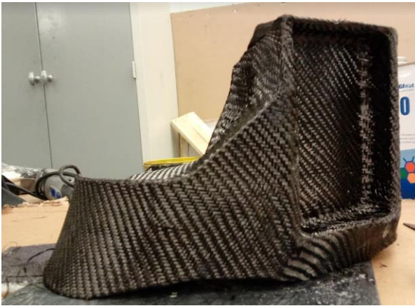
Figure 45. The back brace and femoral links being manufactured.
