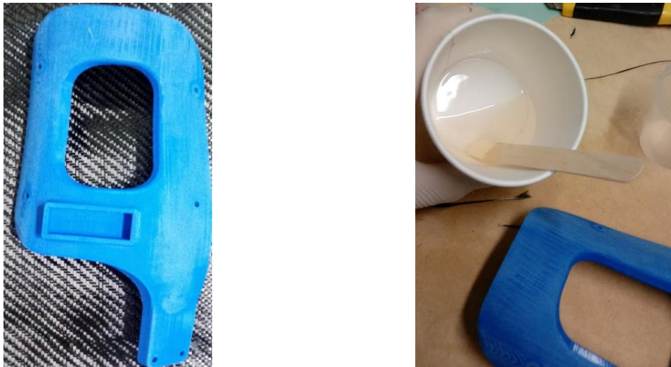
Figure 42. 3D-printed parts being prepared for carbon fiber laying.
