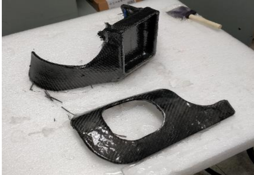
Figure 46. The back brace and femoral link immediately after the completion of the carbon fiber lay up.
